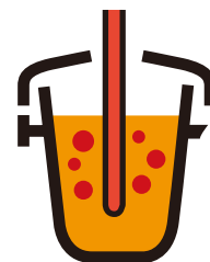
盛鋼桶吹射及攪拌處理 Ladle Injection Station & Stirring
